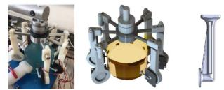
Fig. 14. Left: Photograph of the experimental system. Center: drawing of the experimental system setup. Right: L-shape stem with square toe fixed of the plate of vibrators in order to generate a shear wave source condition.
