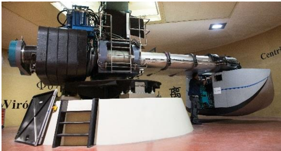
Figure 1 : 200×g-tons & 5.5m radius IFSTTAR's geo-centrifuge
