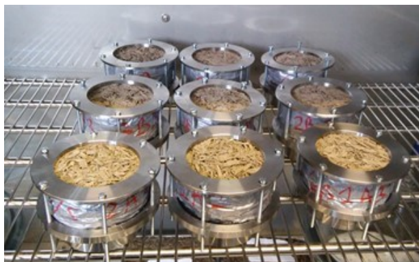
Fig. 4. Typha clay samples for permeability measurements.
