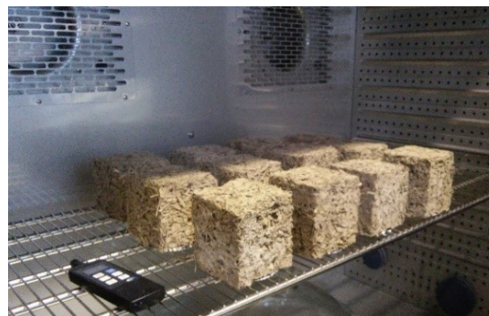
Fig. 5. Typha clay samples for sorption isotherm.
