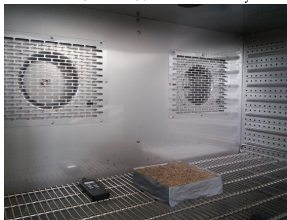
Fig. 6. Typha clay samples for MBV measurements.
