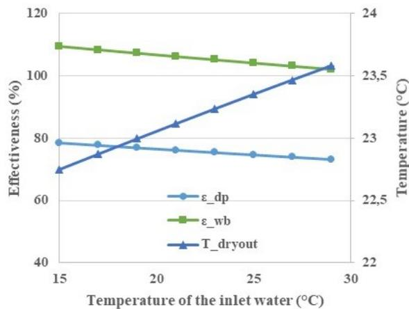
**Fig. 7.** Cooling effectiveness and supply air temperature as a function of water temperature.
