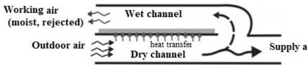
**Fig. 1.** Schematic representation of the studied evaporative dew point cooler.
