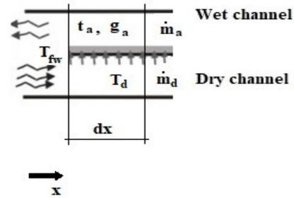
**Fig. 2.** Cross section of the computational element.
