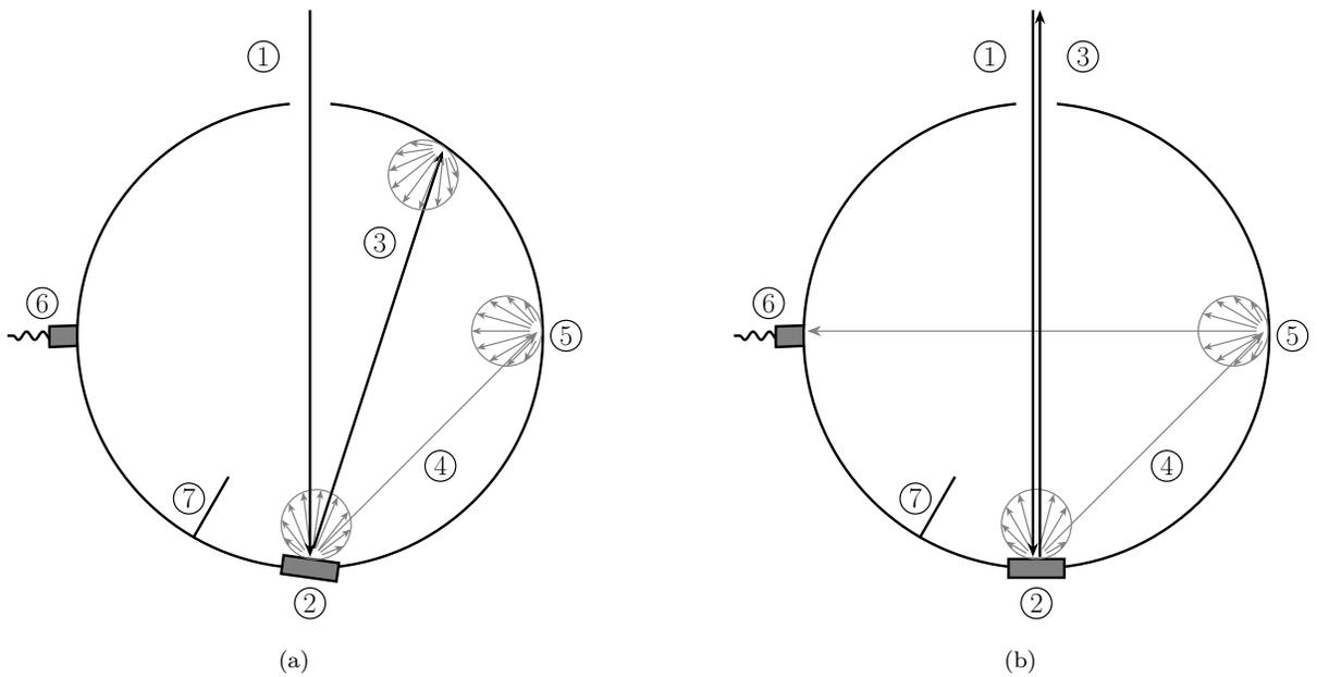
Figure 4: Integrating sphere working principle. (a) diffuse reflectivity measurement, sample tilted at  $3^{\circ}20'$  (b) total reflectivity measurement. (1) incident ray, (2) sample, (3) specular reflected ray, (4) diffuse reflected ray, (5) reflection of the diffuse radiation, (6) detector, (7) baffle to prevent first reflection direct hit on the detector
