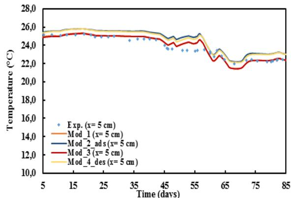
Fig. 10. Comparison between temperature profiles at x = 5 cm.
