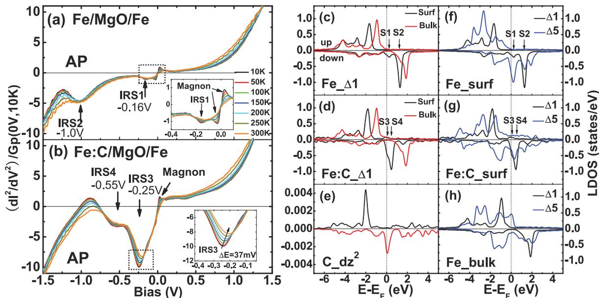
FIG. 1. (Color online)  $d^2I/dV^2$  curves measured at different temperatures in an AP configuration for MTJs (a) without C and (b) with C. The insets show the magnified zoom in the dashed square. LDOS in  $\Delta_1$  symmetry for bcc Fe(001) slabs (c) without C and (d) with C. (e) LDOS in  $d_{z^2}$  symmetry for surface C. Comparison of LDOS in  $\Delta_1$  and  $\Delta_5$  symmetry for surface Fe layer (f) without C, (g) with C, and (h) bulk Fe.
