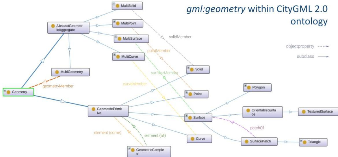
Figure 2. CityGML 2.0 Ontology: Geometry Classes and Properties [8]
