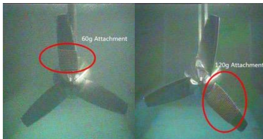
Figure 11. Different imbalance fault severities setting on the MCT blade.
