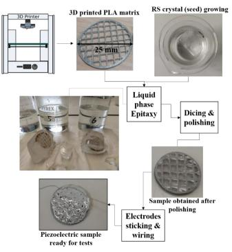
FIGURE 1. Illustration of the manufacturing process flow of the RS/PLA piezoelectric samples (diameter 25 mm, thickness: 2.5 mm).
