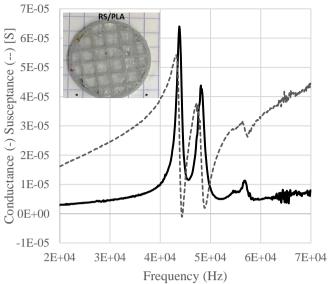
FIGURE 2. Conductance and susceptance spectra of 2.5 mm thick RS/PLA manufactured sample.
