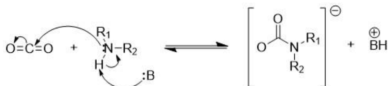
Scheme 15 : Amine carbonation mechanism 111
