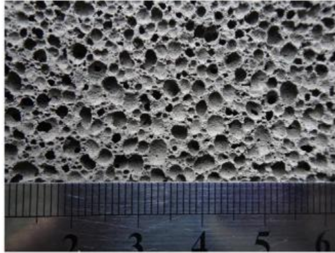
Figure 3: Geopolymer foam obtained by Feng et al. 47 (conditions: 80 g of water, 55°C, 6g of H 2 O 2 )
