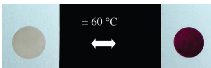
Figure 26. Thermochromic effect of the liquid crystal film [\text{Fe}(\text{C}_{12}\text{-trz})_3](4\text{-MeC}_6\text{H}_4\text{SO}_3)_2 . [119]
