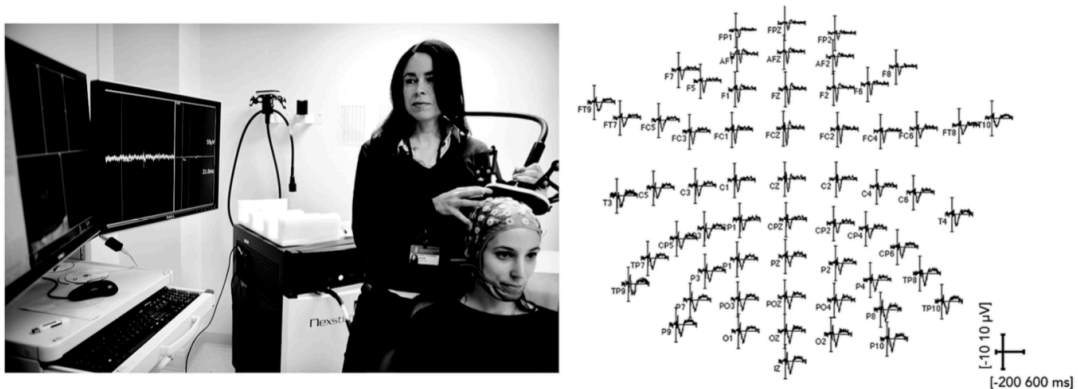
FIGURE 7 Transcranial magnetic stimulation (TMS) combined with electroencephalography (EEG). Left : a TMS-EEG system (Nexstim Oy, Helsinki, Finland). Right : TMS-evoked potentials for individual EEG channels.
