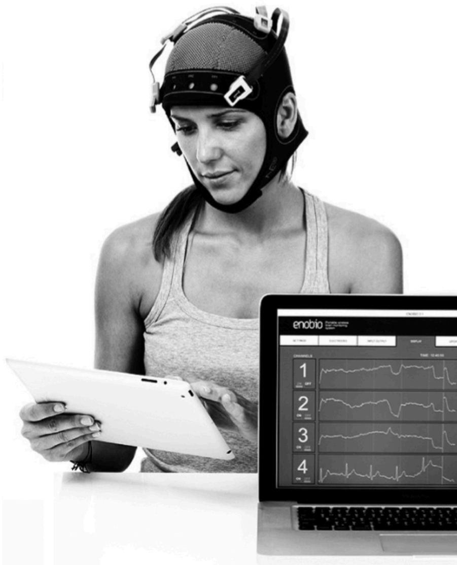
FIGURE 2 Setup of a wearable, modular, and wireless system of electroencephalography (EEG) recording (ENOBIO, Starlab, Barcelona, Spain).
