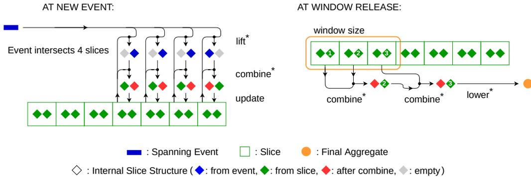
■ **Figure 5** Usage of functions lift\*, lower\* and combine\* to insert events and release aggregates in SES with cumulative aggregate functions. The Internal structure is duplicated to keep track of: the events which end in the slice  $\phi$  on the left, and the events which end after the slice  $\varphi$  on the right.
