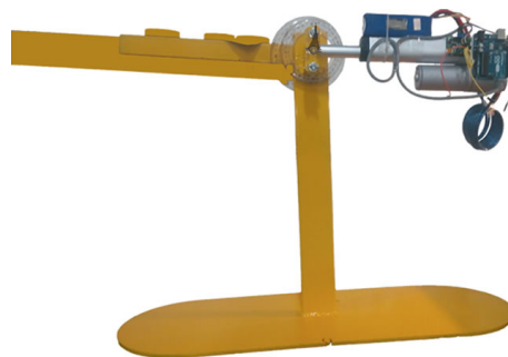
Fig. 8. Mobile mass test bench. It is used for finding a first relation between the radio of the actuator, the mobile mass and the angle of inclination of the test bench.
