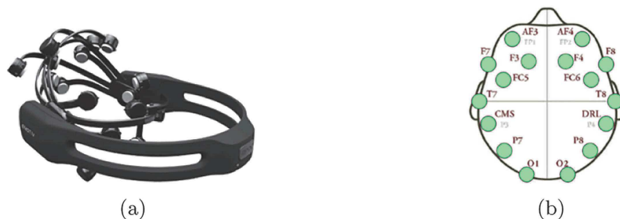
Fig. 2. (a) Emotiv EPOC+ helmet, (b) Location of the Emotiv EPOC+ helmet electrodes (10–20 International Standard).
