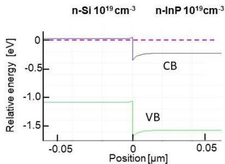
Figure 1: Band diagram (Conduction Band and Valence Band) calculated by Lumerical CHARGE solver . Doping are n-Si/ n-InP both  $10^{19}\text{cm}^{-3}$
