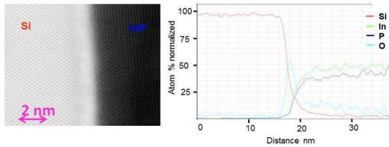
Figure 2 : O<sub>3</sub> activation bonded interface
