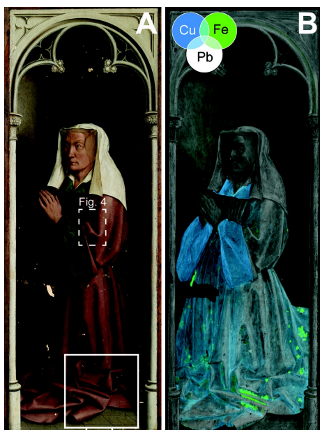
Figure: A) Donor portrait of Elisabeth Borluut. B) Composite elemental image showing the distribution of copper (blue), iron (green), and lead (white).
