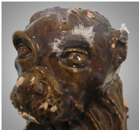
Figure: Unknown efflorescence needles on the eyebrow and the ear of a glazed terracotta lion head, 17th c., E3768, Landesmuseum Württemberg, Stuttgart (Marian Schüch 2015)
