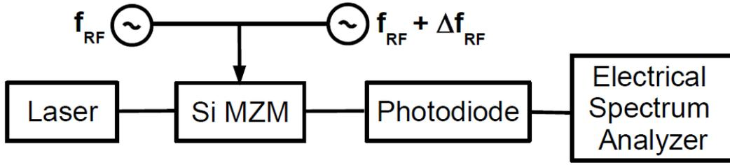
Figure 2. Generic schematic of the dual-tone method setup. Two RF signals at frequencies  $f_{RF}$  and  $f_{RF} + \Delta f_{RF}$  are mixed together before being applied to the modulator. Si MZM: Silicon Mach-Zehnder modulator.
