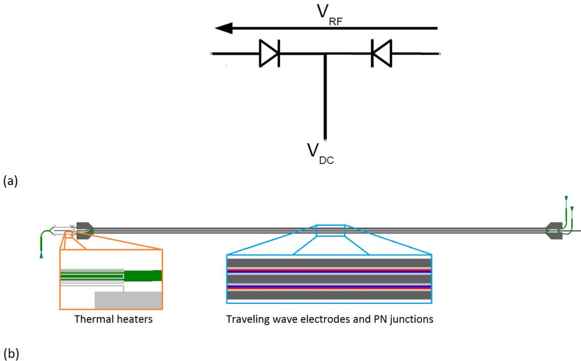
Figure 1. (a) Generic electrical scheme of the modulator.  $V_{RF}$  is the applied RF voltage and  $V_{DC}$  is an electrical DC potential applied to reverse bias both diodes. (b) Schematic top view of the silicon MZM arms. The two highly-doped N regions are connected to the same metallic strip. The insets provide details of the thermal heaters and the PN junctions.
