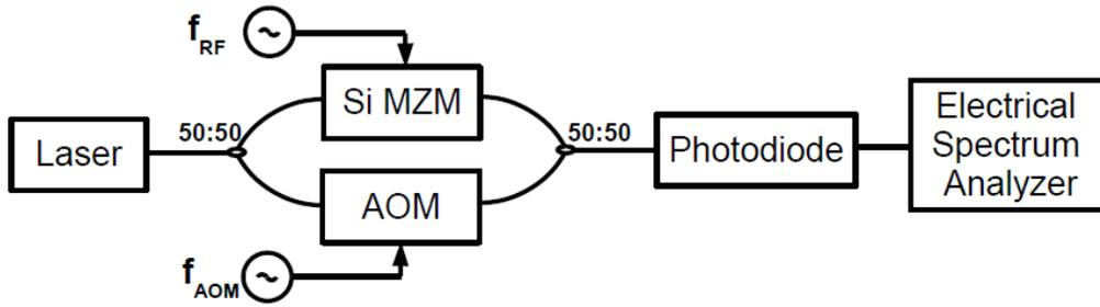
Figure 4. (a). Generic schematic of the experimental setup required for the acousto-optic modulator-based method. A Single RF tone with a  $8V_{pp}$  amplitude and a frequency of  $f_{RF} = 2\text{GHz}$  is applied to the silicon modulator, while the external acousto-optic modulator is driven with a  $f_{AOM} = 40\text{ MHz}$  signal. AOM: Acousto-optic modulator. Si MZM: Silicon Mach-Zehnder modulator.
