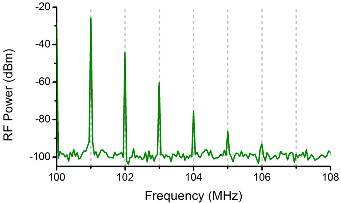
Figure 3. Experimentally measured electrical spectrum when two RF signals of  $3 V_{pp}$  and frequencies of 100 and 101 MHz are mixed before being applied to the silicon modulator. Beat-notes emerge over the noise floor from 100 MHz to 106 MHz.
