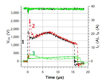
Fig. 12: Failure of the 10 kV-class SiC BJT after 2 repetitive short-circuit events 1 s apart. The dotted curves stand for the collector current. On the third try the device behaves as a current limiting device.
