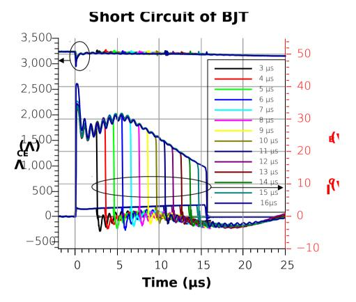
Fig. 10: Short-circuit ruggedness of the 10 kV SiC BJT. No degradation or failure was observed even at 16 µs duration
