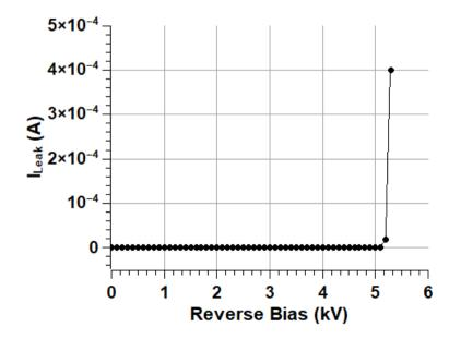
Fig. 2: The measured breakdown voltage of the 10 kV-class SiC BJT.
