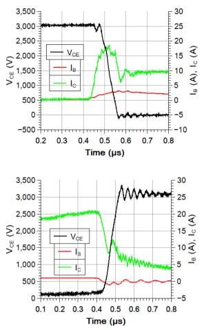
Fig. 8: Switching waveforms of 10 kV SiC BJT. Full wave (up), turn-on (left), turn-off (right)
