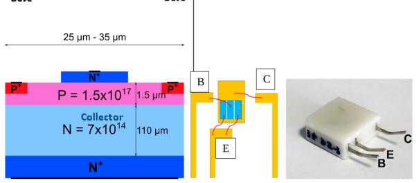
Fig. 1: The elementary cell pitch, the internal connection schematic and the finished packaged device from left to right.
