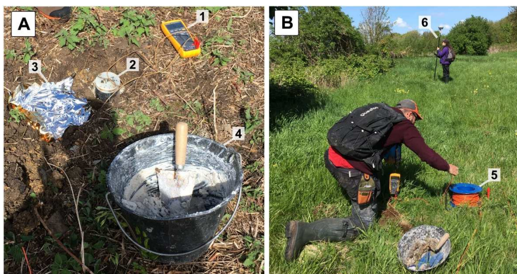
289 290 Fig. 6 – Self-potential device: (A) Derivation control between fixed and mobile electrode 1. High-impedance multimeter; 2. 291 Mobile electrode; 3. Fixed electrode protected by the silver side of a survival blanket (to reflect solar radiation and limit the 292 thermal drift). The blanket is then covered with clumps of earth during the survey; 4. Bucket with bentonite slurry. (B) 293 Measurements of SP anomaly in the sliding area. 5. Cable reel connecting both electrodes; 6. GNSS acquisition to localize 294 SP measurements.
