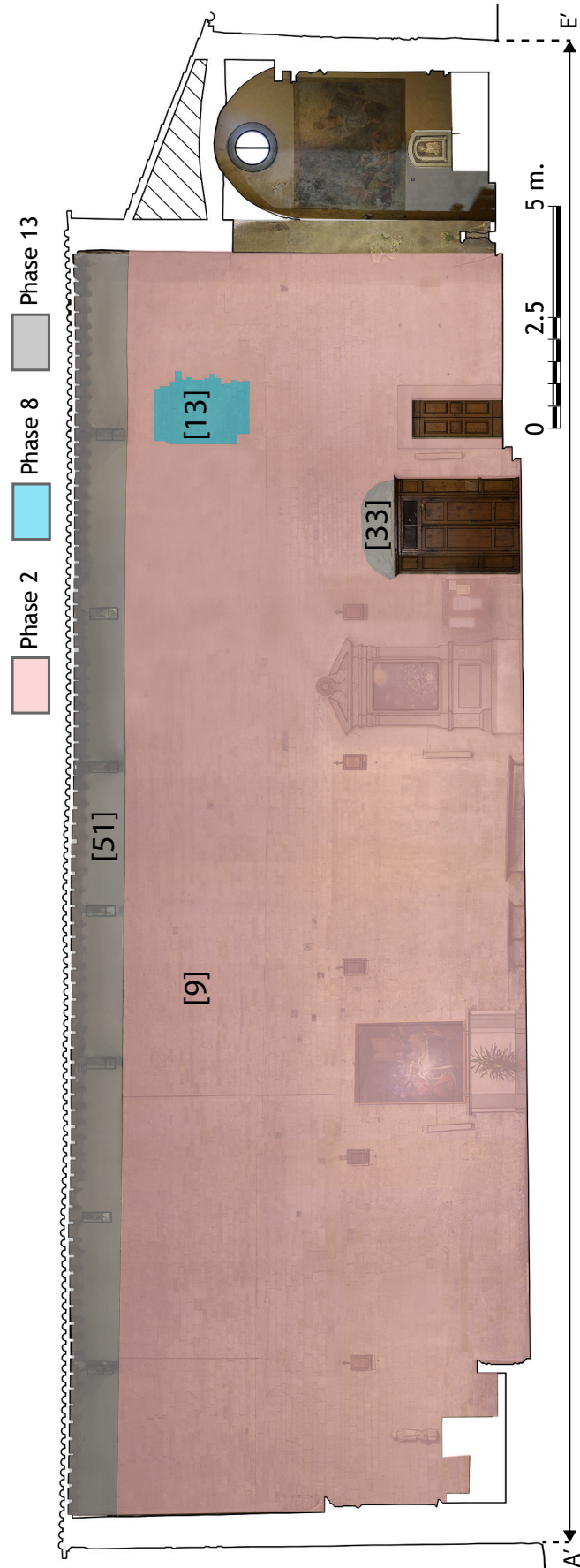
Figure 11: Stratigraphy of the internal north-facing of the church (MR14) including the nave (on the right), the bell tower (on the middle) and the north lateral chapel. Phase 2, phase 4, phase 7, phase 8, and phase 13 are identified.
