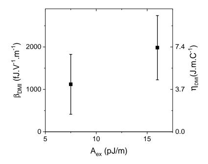
FIG. 4:  $\beta_{DMI}$  coefficients deduced from the experimental  $M_s$ , t,  $L_{eq}$  and  $K_{eff}$  values as a function of the chosen  $A_{ex}$  value. The error bars are calculated from the standard error on the slope on a linear fit of D(V).
