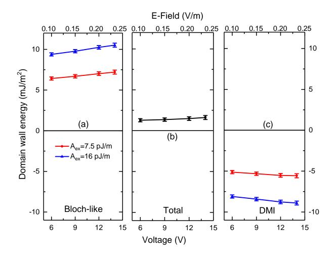
FIG. 3: Different components of the wall energy  $\sigma_w$  as a function of applied EF : (a) Bloch wall energy  $\sigma_w^{Bloch}$ . (b) Total energy  $\sigma_w$ . (c) DMI contribution  $\sigma_w^{DMI}$ .
