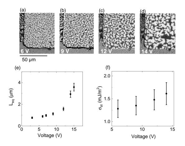
FIG. 2: (a)-(d) p-MOKE images of the evolution of equilibrium stripe width  $L_{eq}$  with gate voltage. (e) Equilibrium stripe width  $L_{eq}$  as a function of gate voltage. We estimated from repeated measurements a ~ 10% error on  $L_{eq}$  due to imperfect demagnetization. (f) Deduced domain wall energy as function of gate voltage. The error bars correspond to a 16% error calculated from the propagation of the errors in  $M_s$ , t and  $L_{eq}$ .
