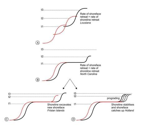
**Figure 8.** (colour) Diagram of barrier-shoreface retreat mode. A. Barrier and shoreface retreat at equal rates (keep-up). B. Shoreface retreat slower than barrier C&D. Shoreface "catch-up" with t1 t2 t3 the successive stages of sea level rise. From Cooper et al. (2018)
