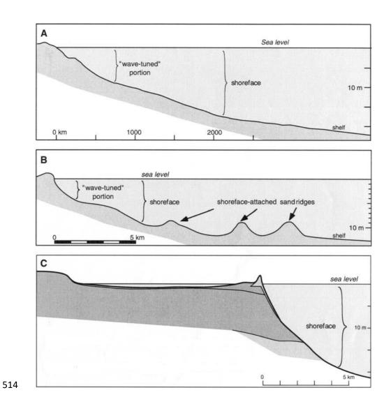
**Figure 5.** Diagram of various possible shoreface morphologies (Modified from: Clifton et al., 2005) A: Unconstrained morphology B: Morphology influenced by sediment features C: Morphology constrained by geologic framework (thin layer of sand over bedrock)
