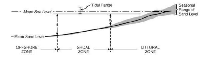
**Figure 3.** Definition of inner and outer depth of closure (Hallermeier, 1981) with dI the inner depth of closure (DoC) and di the outer depth of closure or wave base. Here, the littoral zone corresponds to the upper shoreface and the lower shoreface is included in the shoal zone.
