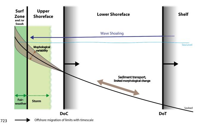
**Figure 9:** Definition of the shoreface, showing upper and lower shoreface limits. The surf zone is represented in dark green, with light green areas in the upper shoreface representing episodic expansion of the surf zone during energetic events. Brown arrows depict bidirectional movement of sediment in the shoreface and resulting morphological variability.
