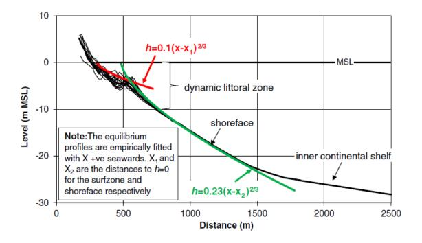
**Figure 2**.(colour) Example of equilibrium profiles fitted for the surf zone and shoreface on the Australian Gold Coast (from: Patterson and Nielsen 2016). In this example, the dynamic littoral zone equates to the surf zone and upper shoreface.
