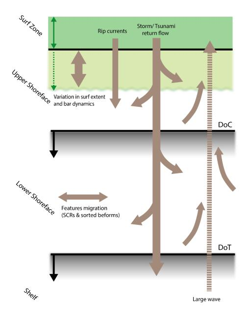
**Figure 7:** Schematic representation of sediment exchange over the shoreface. With, The surf zone (in dark green) and upper shoreface (light green) are depicted with the upper and lower shoreface limits (solid black lines; see Figure 9) The schematic represents episodic expansion of the surf zone during energetic events. In brown, the arrows depict the sediment transport mechanisms across the shoreface.
