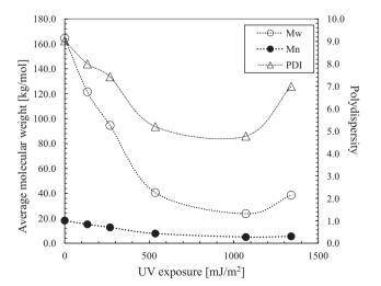
**Fig. 1.** Evolution of the number average,  $M_n$  and weight-average,  $M_w$  molecular weights and the molecular weight distribution (PDI =  $M_w/M_n$ ) as a function of the UV emitted dose.
