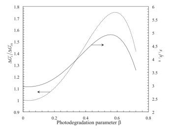
Fig. 5. Evolution of the normalized activation energy and the normalized initial shear strengths.
