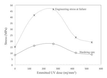
**Fig. 4.** Effect of photo-degradation on the engineering stress at failure and the hardening rate.
