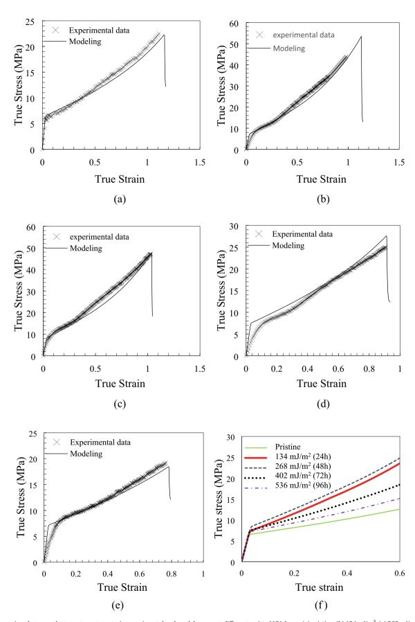
Fig. 6. Comparison between the true stress-true strain experimental and model curves at different emitted UV doses: (a) pristine, (b) 134 mJ/m², (c) 268 mJ/m², (d) 402 mJ/m², and (e) 536 mJ/m² finally (f) presents the predicted true stress-true strain curves of the all the photo-degradation conditions.
