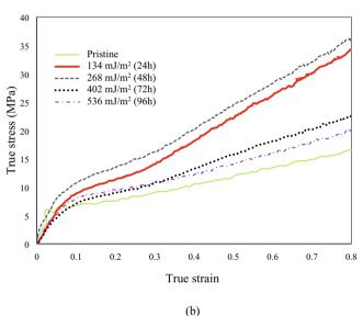
**Fig. 2.** As-received and aged materials at different UV emitted dose (a) Engineering stress-engineering strain plots (b) True stress-true strain curves; the inset presents the geometry of the tensile specimen, dimensions in mm.
