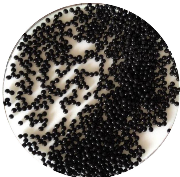
Fig. 1. Magnetic alginate beads.
