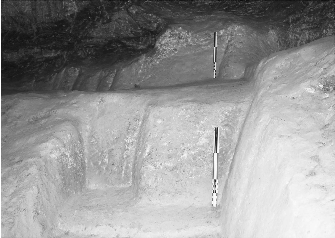
Figure 9. Laurion. Mégala Pefka sector. Mi 7 – Underhand stoping technique
