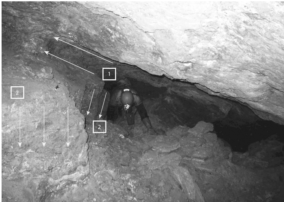
Figure 13. Laurion. Spitharopoussi plateau. Spi 18 – Deep works in the Third Contact. Mining technique process using a horizontal cut to the roof. To the right, behind the working face, a cluster of mineralised blocks. 1. Horizontal mining. 2. Vertical mining
