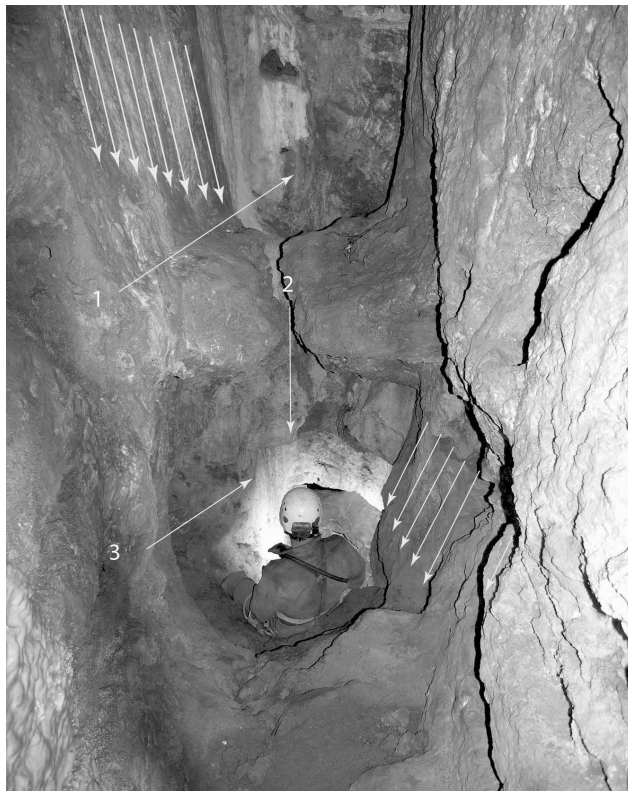
Figure 16. Spitharopoussi Plateau. Spi 15 – Nyphitsa network. Downward stoping process by benching (rebor-ing) the original gallery. 1. Original 1 st research gallery. 2. Remain of 1 st gallery floor. 3. 2 nd gallery
