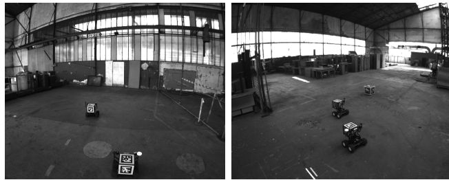
Fig. 1: Screenshots of inter-robot direct observations between the drone and ground robots outfitted with AprilTag markers
