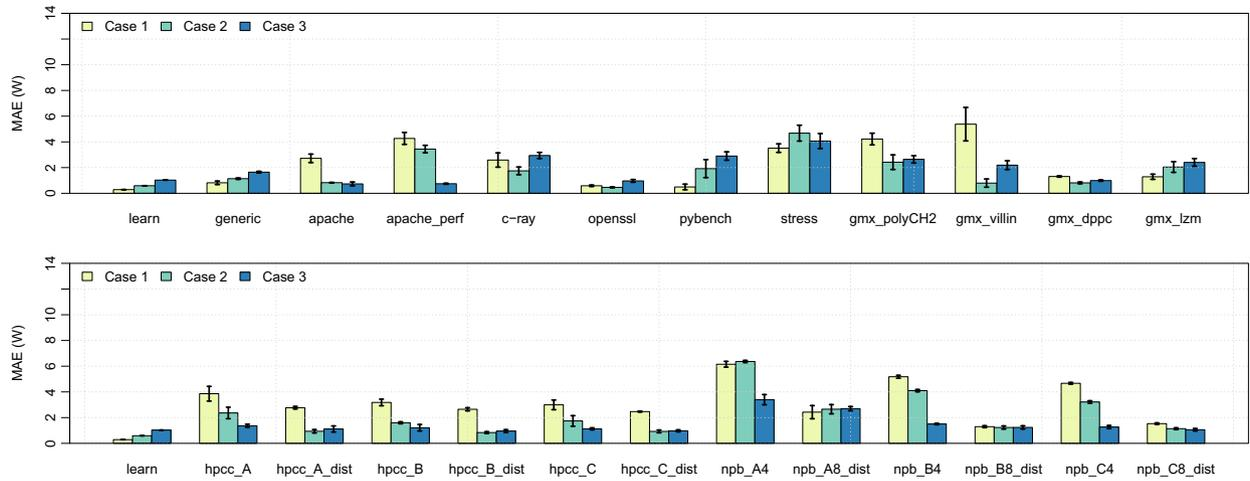
**FIGURE 13** Residual's based reduced ANN power models' comparison for each learning case after workload reexecution. Case 1 has been obtained with a learning based only on the *generic* benchmark; Case 2 with a selection of benchmarks; Case 3 with all benchmarks
