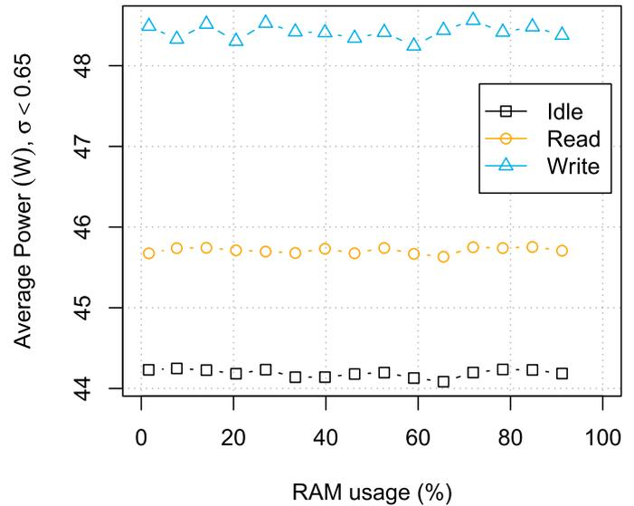
allocation. The minimum and the step size of memory allocation are 60 Mb to 14 Gb with 1 Gb step. The memory allocation was tested with three cases: read, write and idle (no access to the RAM). All these cases kept one core of the system busy, that is, 25 % of processor usage for i7 while being at maximum frequency.
