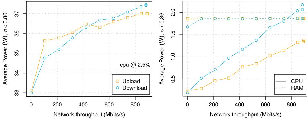
**FIGURE 7** Network usage impact on the overall power consumption for Gigabit Ethernet cards. On left, reference of maximum power consumption on cpu-related benchmark at 2.5% load is shown. On right allocated memory is shown as being constant and processor is shown to stay under 2% during the whole experiment
