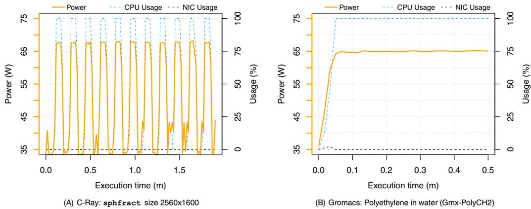
**FIGURE 9** Multithreaded (four cores) CPU intensive workloads' profiles
