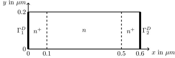
FIGURE 3. Geometry of the  $n^+nn^+$  ballistic diode.
