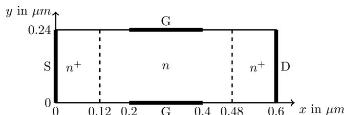
FIGURE 9. Geometry of the double-gate MESFET device.
