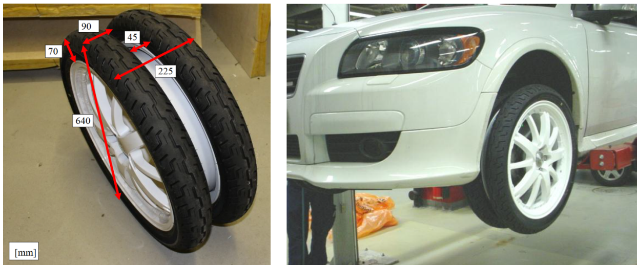
Figure 4-20 Dimensions (in mm) of the DualQ tyre prototype (left) and DualQ tyre prototype mounted on the test vehicle during the CITYHUSH project (right) [71].
