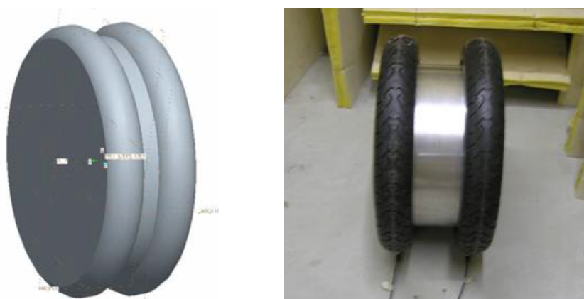
Figure 4-11 The concept of Twin-tyre (left) and Twin-tyre mock-up developed during the QCITY project [67].
