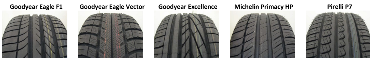
Figure 4-8 Five tyre models of dimensions 225/45 R17 used for CPX noise measurements in [65].
