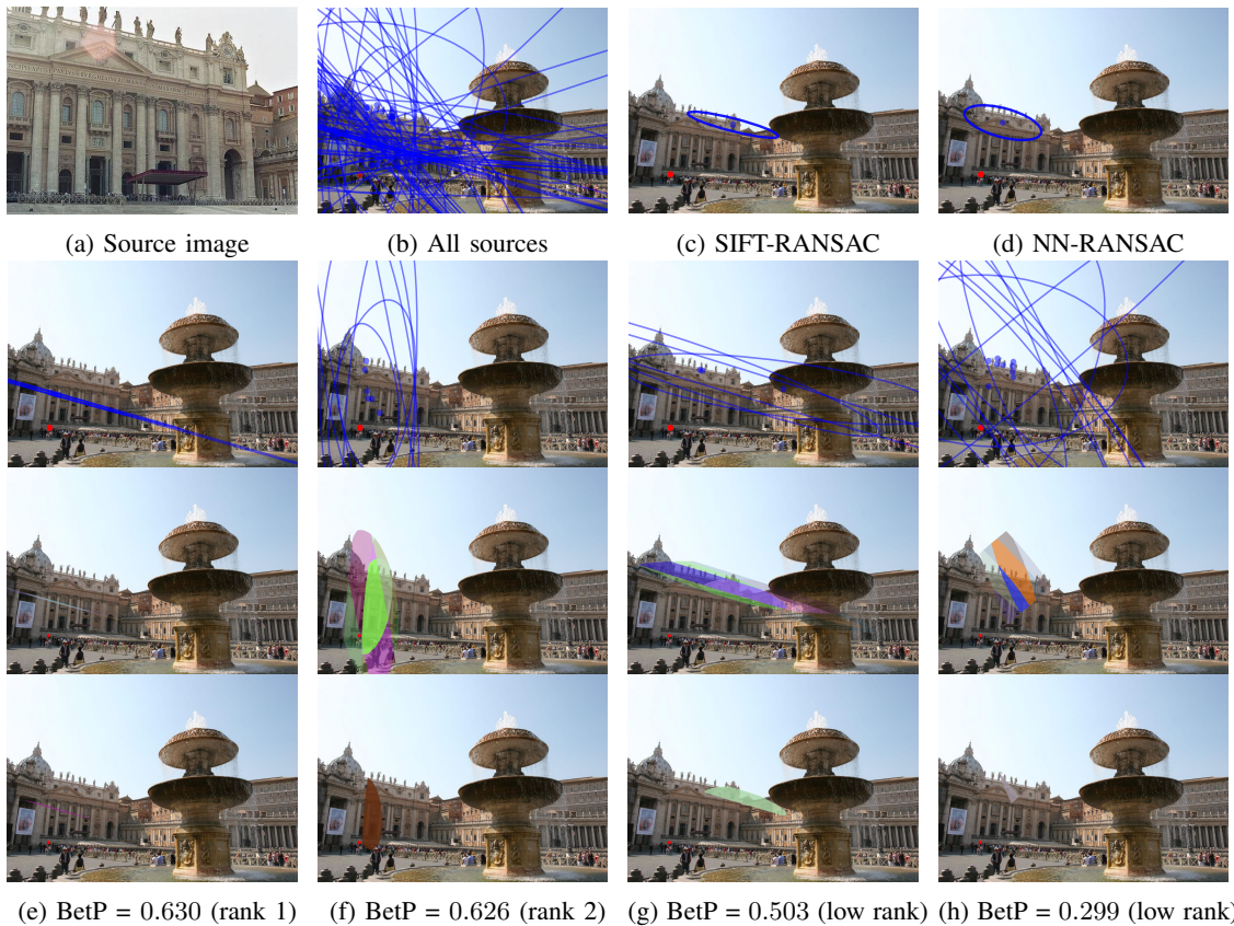
Fig. 2: Qualitative illustration of our method. Upper row: the source image (a), set of epipole uncertainty ellipses (b) and the result of existing methods (c)-(d) (the ground truth is highlighted in red). (e): the top ranked cluster (ellipses, final BBA and BetP). (f): the second ranked cluster. (g)-(h): two clusters with a low rank/BetP due to the sources being less consistent.
