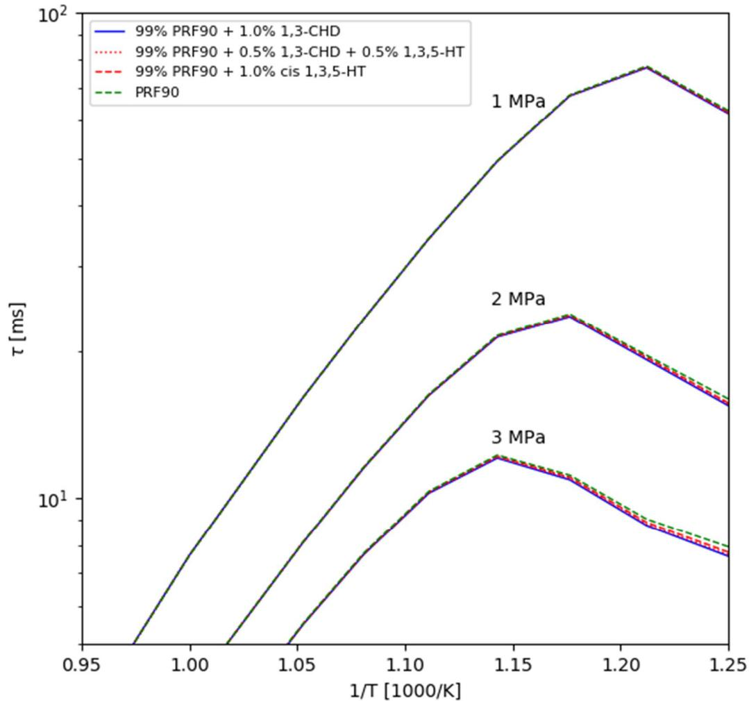
**Figure 12.** Constant pressure ignition delay for 1 % 1,3-CHD and 99 % PRF-90, 1 % 1,3,5-HT and 99 % PRF-90 and a 50% mixture of these two at  $\Phi = 0.5$ .
