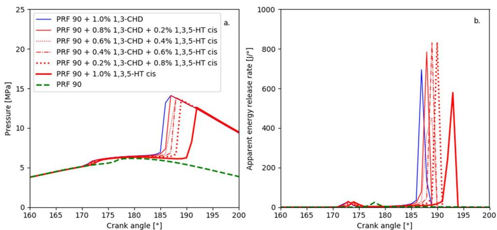
**Figure 9.** Influence of photochemical isomerisation reaction on cylinder pressure (a.) and apparent energy release rate (b.) of the engine cycle. HCCI engine operating conditions: Constant engine speed of 2000 rpm and  $\Phi = 0.50$ . Highest engine load 1.15 MPa IMEP for 99 % PRF-90 + 1.0 % 1,3-CHD.
