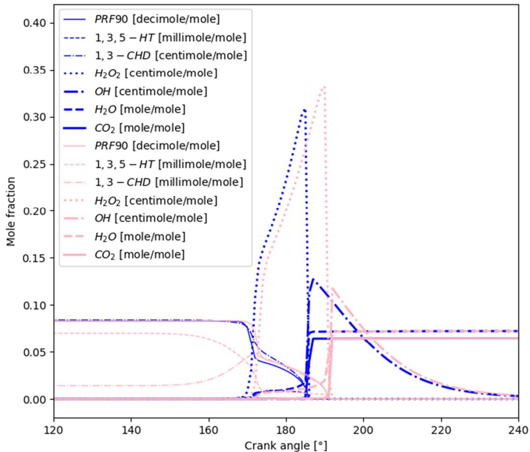
**Figure 11.** Species mole fraction development for 1 % 1,3-CHD and 99 % PRF-90 (blue lines) and 1 % 1,3,5-HT and 99 % PRF-90 (red lines). Equivalence ratio  $\Phi = 0.5$  and HCCI engine speed  $\omega = 2000$  rpm.
