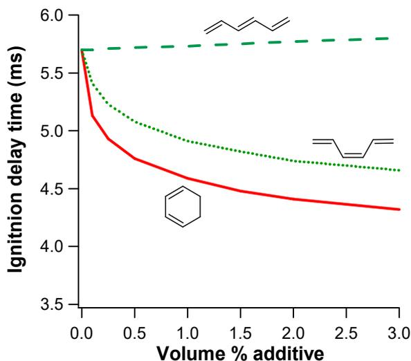
**Figure 8.** Ignition delays of PRF90 as a function of volume percent additives: 1,3-CHD (solid line), *cis*-1,3,5-HT (dotted line), *trans*-1,3,5-HT (dashed line). Conditions: equivalence ratio of 0.4, temperature and pressure of 827 K and 40.1 atm.
