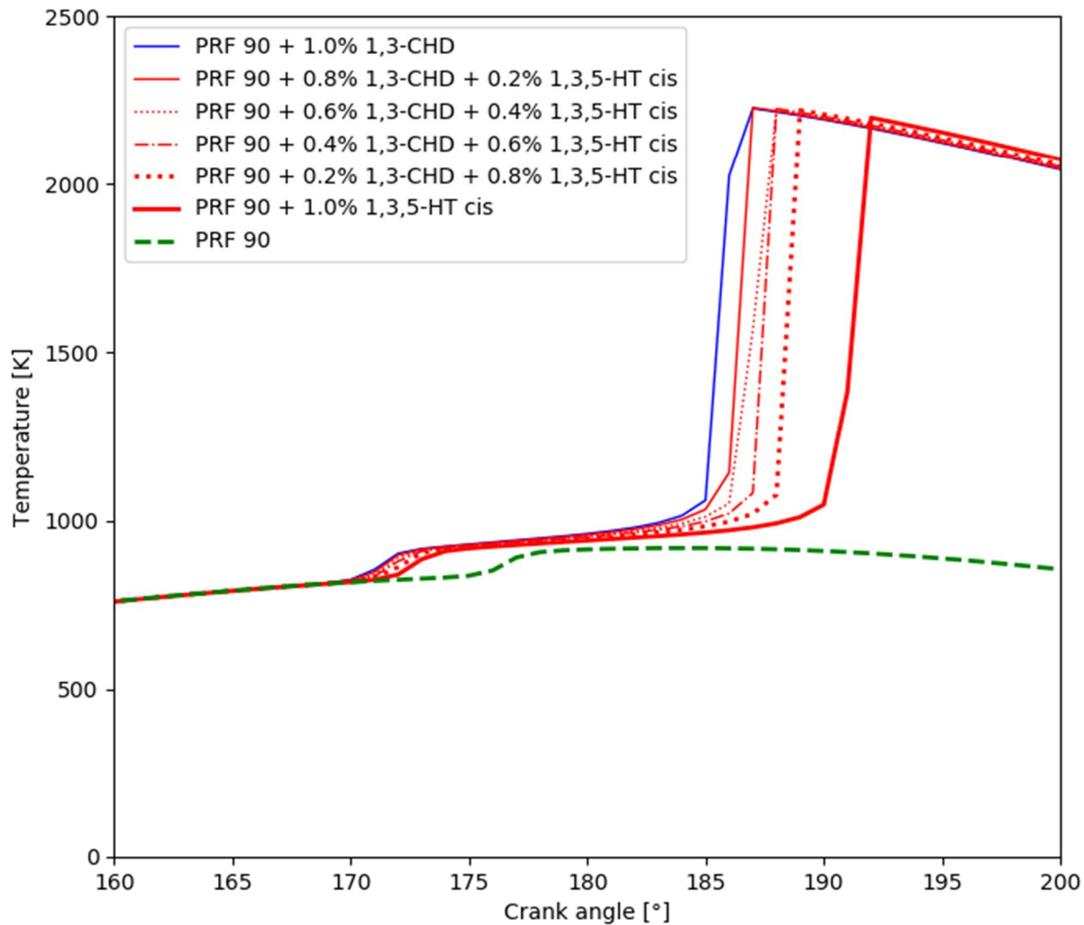
**Figure 10.** HCCI global cylinder temperature at constant engine speed of 2000 rpm and  $\Phi = 0.50$ . Highest engine load 1.2 MPa IMEP for 99 % PRF-90 + 1.0 % 1,3-CHD.
