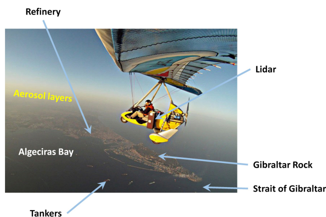
Figure 1. Ultralight aircraft (ULA) above the Strait of Gibraltar. The lidar is located on the left side of the ULA in nadir-shooting position. The aerosol layer can be seen in ochre on the horizon of the photo.
