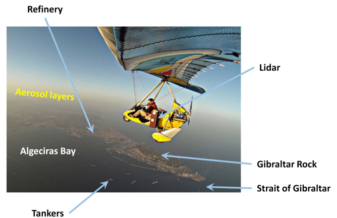
Figure 1. Ultralight aircraft (ULA) above the Strait of Gibraltar. The lidar is located on the left side of the ULA in nadir-shooting position. The aerosol layer can be seen in ochre on the horizon of the photo.
