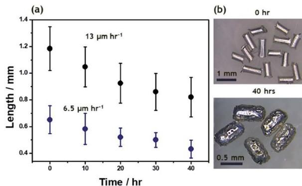
Fig. 1 (a) Average length of Mg wires as a function of electrolysis time at constant  $\varepsilon = 15 \text{ V cm}^{-1}$ , for two different initial sizes:  $1.2 \pm 0.2 \text{ mm}$  (black dots) and  $0.6 \pm 0.1 \text{ mm}$  (blue dots). (b) Optical pictures of Mg wires with an initial length of  $1.2 \pm 0.2 \text{ mm}$  before and after 40 h of electrolysis in a  $5 \text{ mM H}_2\text{SO}_4/\text{ethanol}$  solution.
