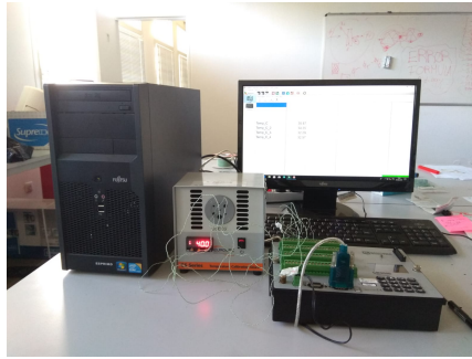
Figure 15: Data acquisition for the calibration tests
