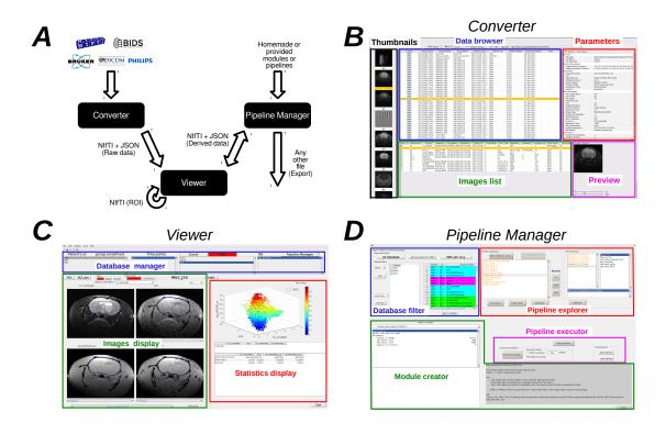
Figure 1: **(A)**: Architecture overview and data flow, **(B)**: Converter, **(C)**: Viewer, **(D)**: Pipeline Manager.
