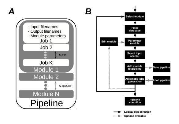
Figure 2: (A): Pipeline architecture, (B): Pipeline creation procedure.
