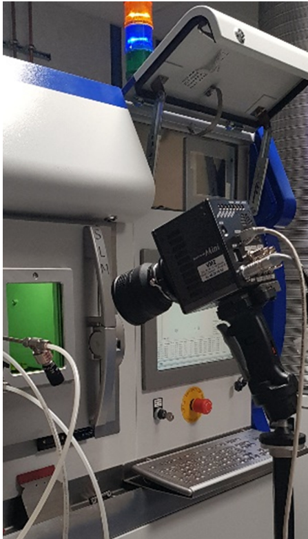
Fig. 6. Photo of the external imaging setup for the SLM 125 machine and image extracted from a low-resolution movie (2000 fps).
