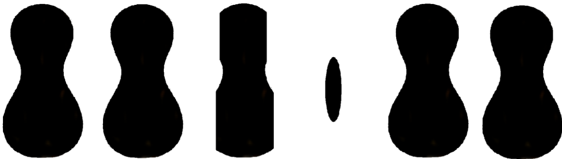
Figure 2: Thickness pattern of the soundboard for TwillC (TwillCA and TwillCB) from left to right: 1 layer Twill-woven AKSACA™ A-38 200 tex (3k), 4 layers of unidirectional Tenax®-E HTS40/12K/HS, 1 layer Twill-woven AKSACA™ A-38 200 tex (3k).
