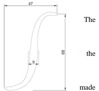
*Figure 3: Design and dimensions of the soundhole for the prototype violins.*
