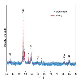
Fig. 1. X-ray diffraction pattern of the sintered  $Mn_{54}Al_{44}C_2$  sample (Co  $K\alpha$  radiation). The tetragonal  $\tau$ -phase Miller indices, traces of a secondary  $\beta$ -phase and a Rietveld refinement profile are shown.
