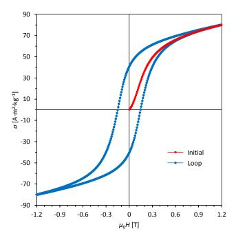
Fig. 2. Initial magnetization curve and hysteresis loop of a heat treated  $Mn_{54}Al_{44}C_2$  powder sample at room temperature.
