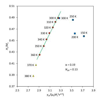
Fig. 8. Relation between the reduced coercive field  $H_c/M_s$  and the reduced nucleus energy  $\gamma_w/(\mu_0 M_s^2 v^{1/3})$  at different temperatures. A linear trend line with fitting parameters are shown.
