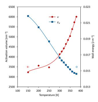
Fig. 6. Experimental activation volume (red) and calculated domain wall energy (blue) as a function of temperature (data points and third-degree polynomial regression).
