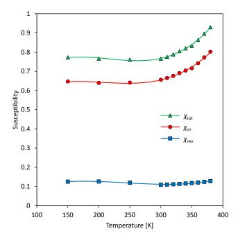
Fig. 4. Reversible (blue), irreversible (red), and total (green) susceptibilities as a function of temperature, measured at near-zero magnetization (data points and third-degree polynomial regression).
