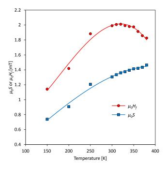
Fig. 5. Temperature dependence of the magnetic viscosity (blue) and fluctuation field (red) derived from the relaxation and susceptibility measurements (data points and third-degree polynomial regression).
