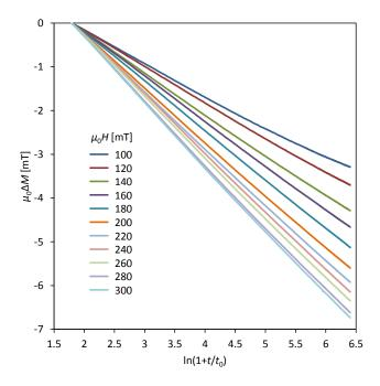
Fig. 3. Magnetization change versus time on a logarithmic scale for different values of the applied field having been reversed (room temperature).
