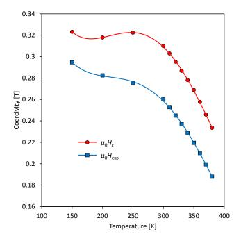
Fig. 7. Measured coercive field (blue) and the coercivity corrected for the fluctuation field (red) as a function of temperature (data points and fourth-degree polynomial regression).
