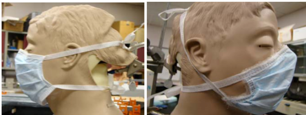
Fig. 13. (a) Unsealed surgical mask in the normal use, (b) sealed surgical mask with crossed straps [86].
