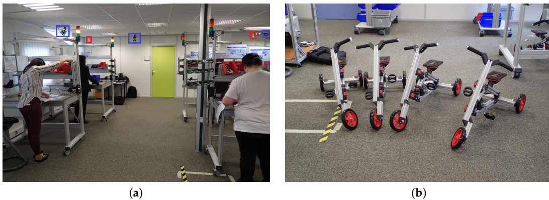
Figure 3. Final assembly of tricycles, and during the process in a NLOS industrial condition made in a workshop. (a) Front view of the assembly process. In the red square is the UWB system and in the blue square is the MoCap system. (b) Result of the assembly process.
