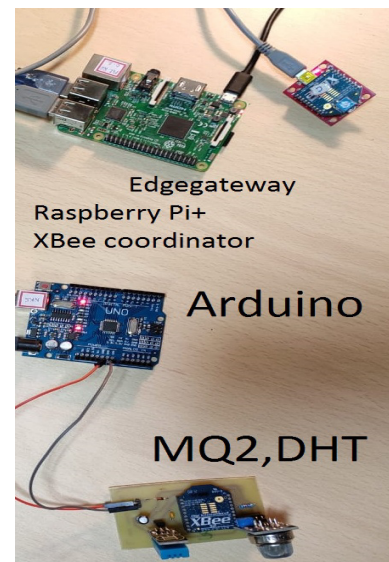
Fig.7 Edge gateway connected with different sensors
