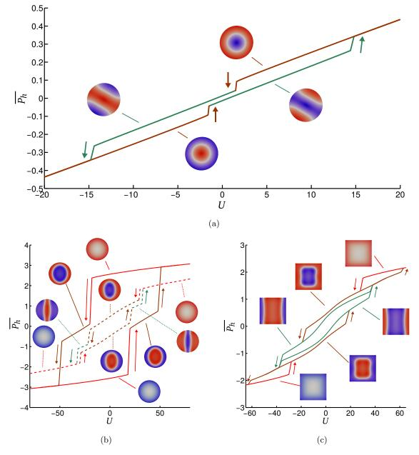
Figure 5: Hysteresis loops from  $\mathcal{T}_h^{(1)}$  with t = -20 (see (a)), from  $\mathcal{T}_h^{(2)}$  with t = -15 (—) and t = -10 (- - -) (see (b)), as well as from  $\mathcal{T}_h^{(3)}$  with t = -10 (see (c)).
