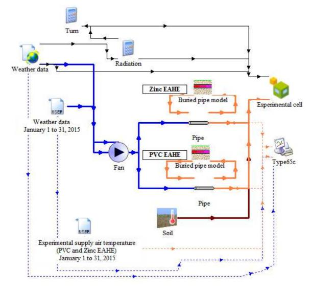
Fig. 9. EAHE models established under TRNSYS.
