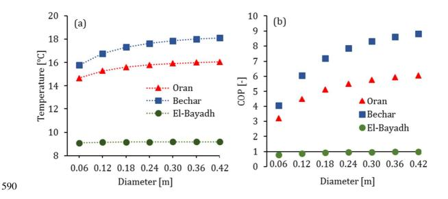
Fig. 26. (a) Air temperature variation at the outlet of the pipe and (b) COP of the EAHE, for different
