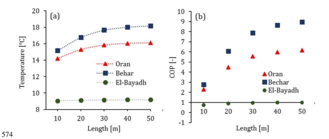
Fig. 25. (a) Air temperature variation at the outlet of the pipe and (b) COP of the EAHE, for different
