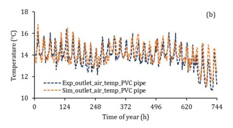
459 Fig. 20. Comparison between experimental and simulated results of the air temperature at the outlet of
