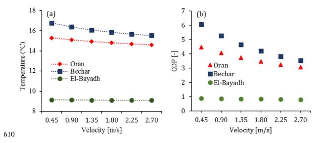
Fig. 27. (a) Air temperature variation at the outlet of the pipe and (b) COP of the EAHE, for different
