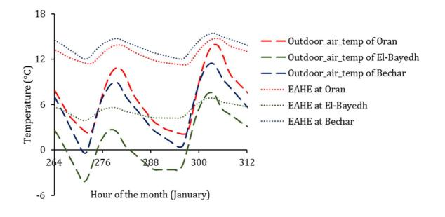
Fig. 22. Air temperature variation at the outlet of the EAHEs for the three sites, viz. Oran, Bechar and
