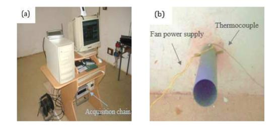
Fig. 7. (a) The acquisition chain and the mini weather station connected to the computer, (b) location of the thermocouple at the outlet of the EAHE.
