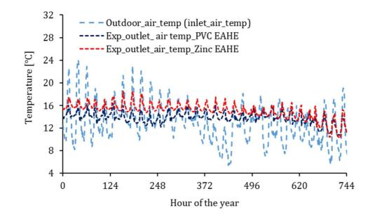
Fig. 12. Experimental measurements of the air temperature at the inlet and outlet of the two PVC and
